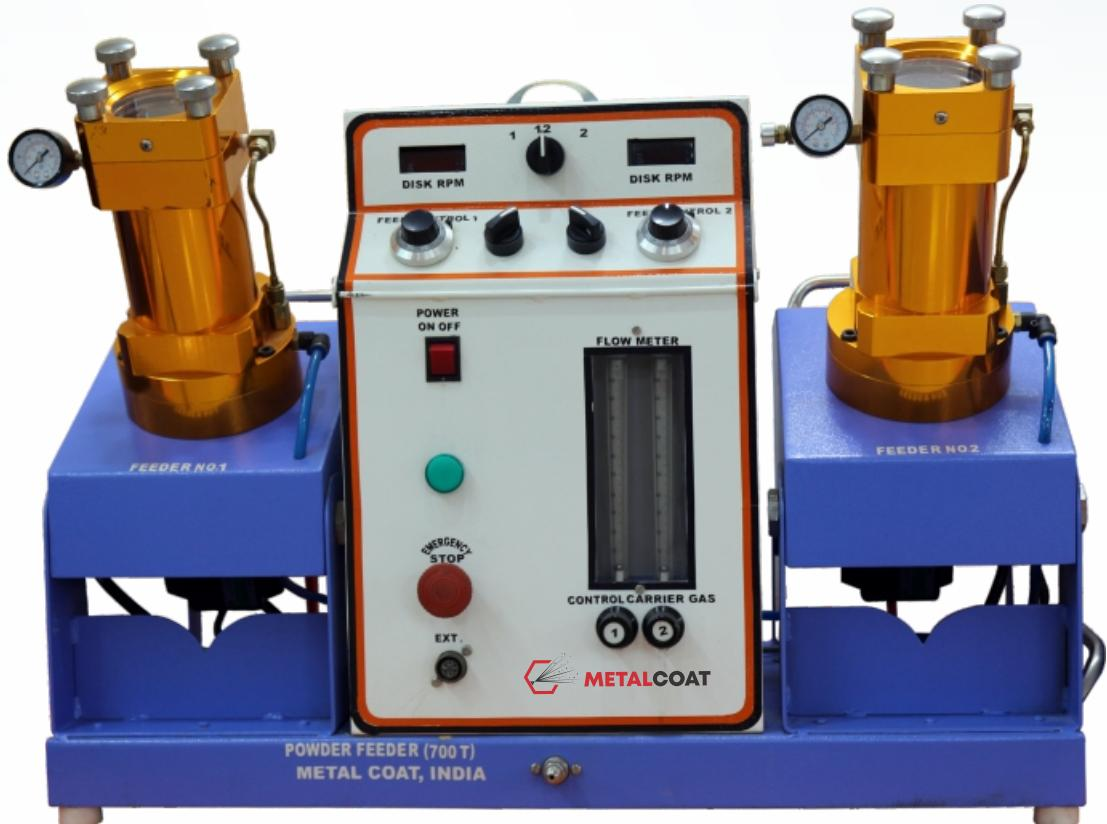
The **MPF 700T (Twin) Powder Feeder** is specifically designed for thermal spray coatings. Its small size makes it a portable powder feeder, which can be carried to site for job work. The unit is controlled to extremely precise and repeatable powder feed rates. The powder hopper (canister) is mounted on a
