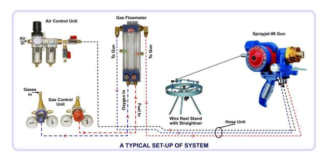
MEC Sprayjet-98-HS system complete with Std. Spares consists of following:-
